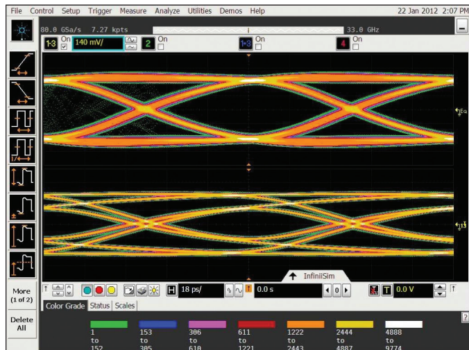
Figure 3 • Receiver equalization techniques such as DFE and CTLE allow the receiver to improve the eye opening.
